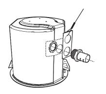
Attach the conduit fitting, safety chain bracket, and lock nut. Install a safety chain/cable (not supplied) that will support up to 16 pounds (7.3 kg).
